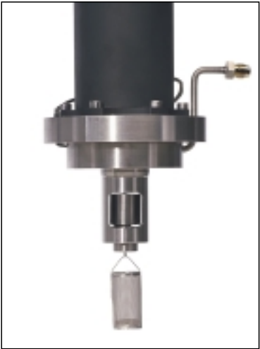
Sorption and density measurement with a magnetic suspension balance (sample basket and titanium sinker)
