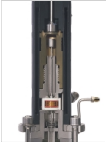
Example of force transmission without contact using a cutaway model of a metal magnetic suspension balance
